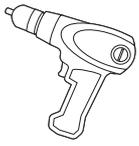
Cordless drill with t25 bit for M6 screw and ph2 bit for wafer head screw.
