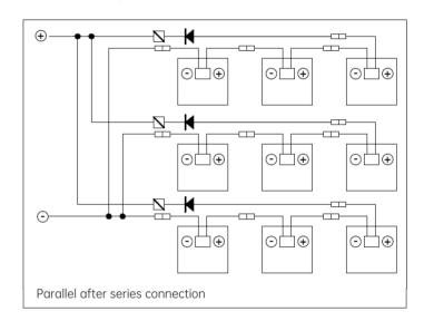
If the PV module is passed through by a reverse current greater than the maximum fuse current of the PV module, the PV module shall be protected with an over current protector of the same specification. If more than two strings are connected in parallel, each PV module string shall be protected with an over current protector as shown above.
