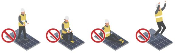
• Do not place heavy objects on the PV module; Do not place the module on a sharp surface. Do not collide or distort the edges of the components.
