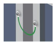
We recommend using the following method to ground correctly, as shown in the figure.
