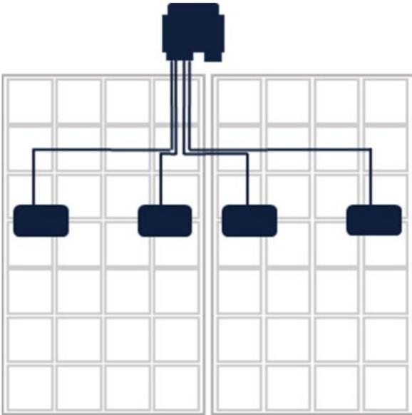
Connecting 2 PV Modules to a dual input commercial Power Optimizer (P800p)
