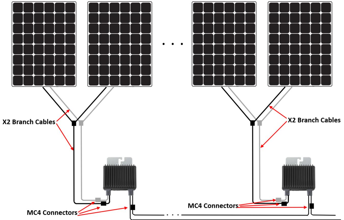
Sense Connect feature supported only at the MC4 connectors at the Power Optimizers short cables.
