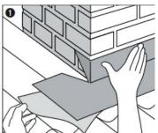
To create a lap joint, join 2 faces of butyl together for an amazing waterproof seal, use the dressing tool or roller to flatten these for presentation purposes.
