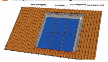
Position the attach angles and the top flashings so that it fits the module thickness. Make cuts on the attach angle at the position of the GSE panel corrugations.
