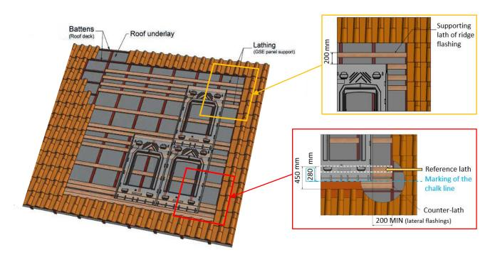
The sections of the support battens are determined according to climatic loads. Use roof battens only if the section is suitable to support climatic loads and if they are positionned according to the GSE battening plan (refer to the online documents)
