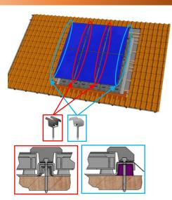
The module is maintained with the upper protrusions and must rest on the pads.
