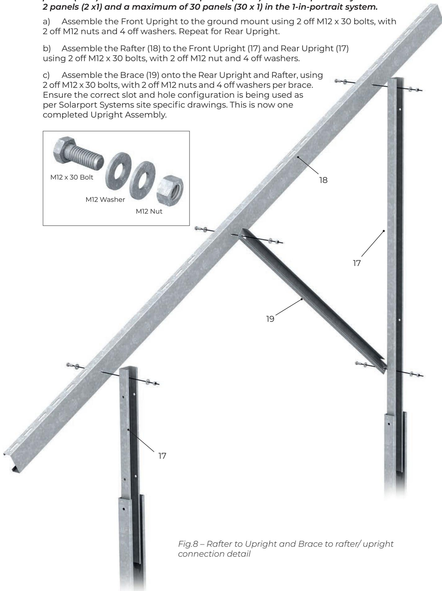
Fig.8 – Rafter to Upright and Brace to rafter/ upright connection detail
