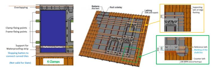
The sections of the support battens are determined according to climatic loads. Use roof battens only if the section is suitable to support climatic loads and if they are positionned according to the GSE battening plan (refer to the online documents)
