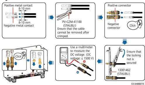
Figure 5-16 Connector connection
