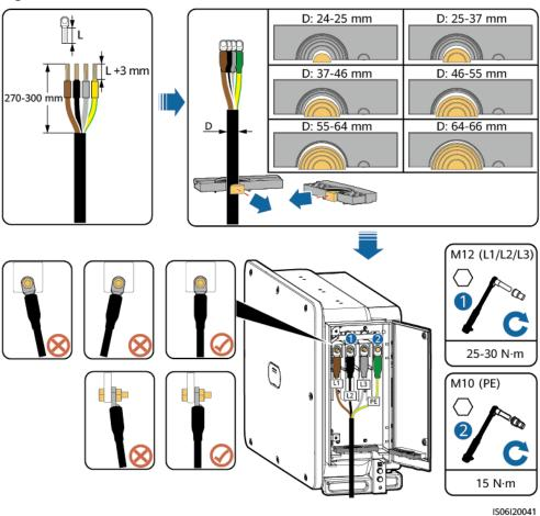
Figure 5-11 Cable connection
