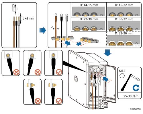
Figure 5-12 Cable connection
