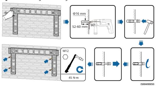
Figure 4-10 Securing the mounting bracket
