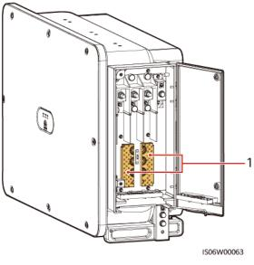
Figure 5-5 Removing the accessories from the maintenance compartment
