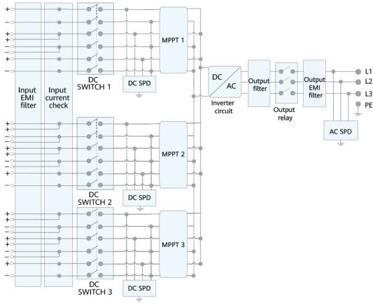
Figure 2-5 Inverter conceptual diagram
