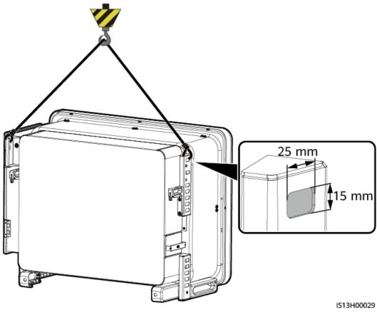
Figure 4-14 Hoisting the inverter
