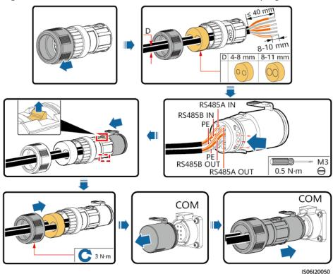
Figure 5-20 Cable connection (4–8 mm two-hole rubber plug)
