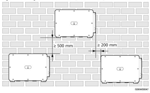
Figure 4-6 Stacked installation mode (not recommended)
