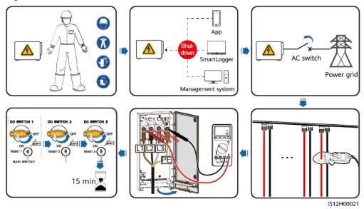
Figure 8-1 Power-off for maintenance
