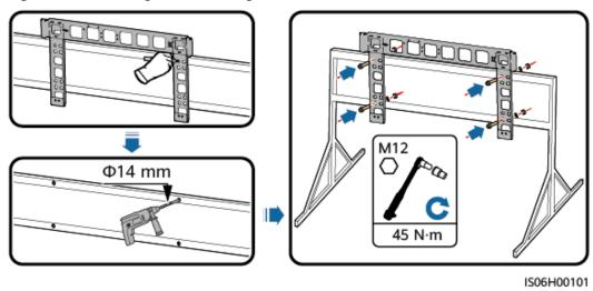
Figure 4-9 Installing the mounting bracket
