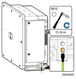
Figure 5-10 Cable connection
