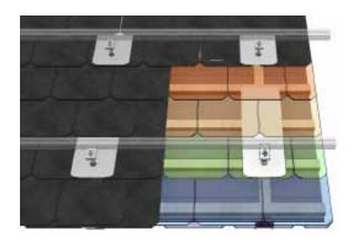
Once the roof inclination has been verified, please ensure that a corresponding variant of the SlatePlan is selected and, notably, that the appropriate overlap distances are observed.
