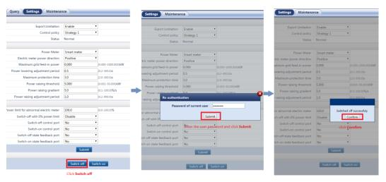
After switch-off is complete, check whether the circuit breaker is OFF.
