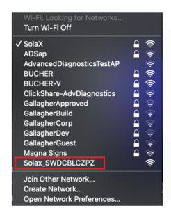
1. With any wireless enabled device such as a laptop, tablet, smartphone etc, navigate to the device settings > Wi-Fi. Here you will see a list of SSID's that are visible, find the SSID Solax\_\*\*\*\*\*\*\*\*\*\*\*\*\*\*\*\* as shown in the screenshot and connect to it.
