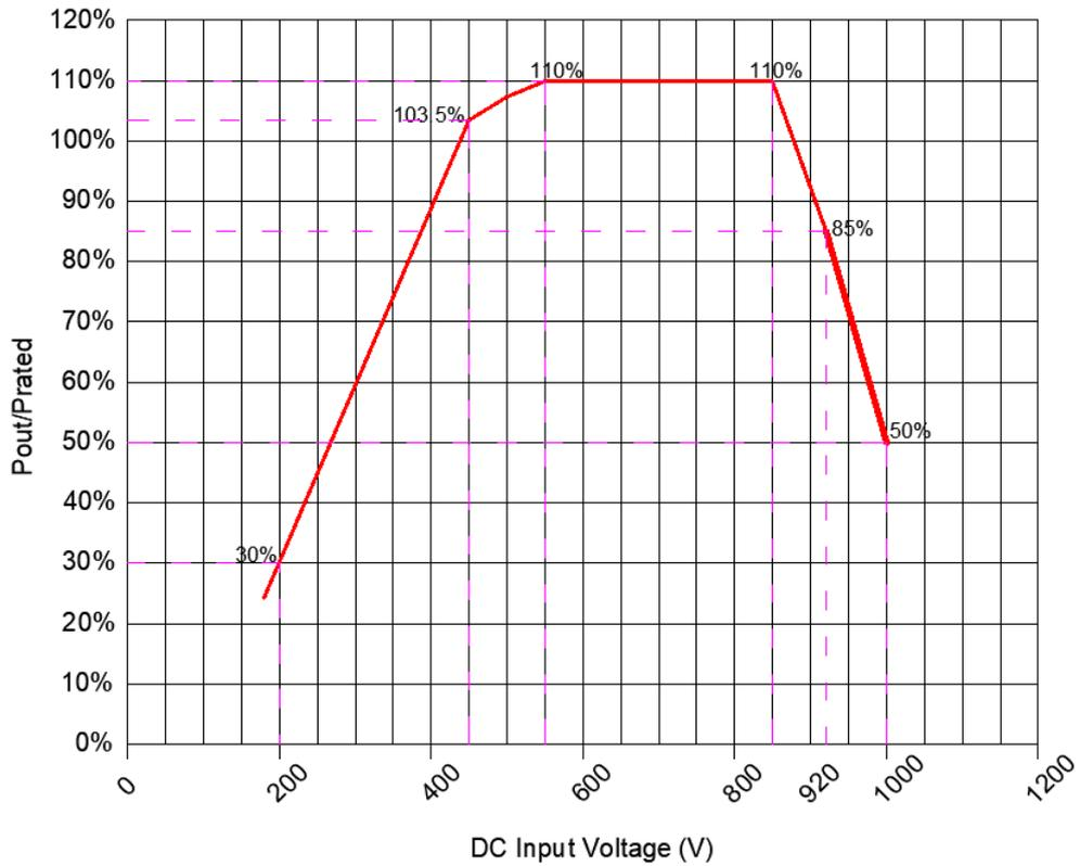
Note: It may differ about 3% because of measurement accuracy and radiation difference. The curve is only for reference.
