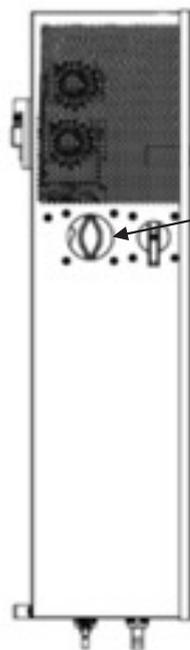
Turn the battery isolation switch to turn on the batteries.
