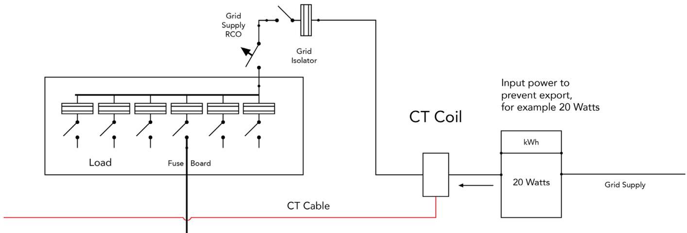
The CT coil is one of the most important parts of the LIFE3.6HYB02. This device reduces the power of the inverter to prevent feeding power to the grid. This is also known as zero export.
