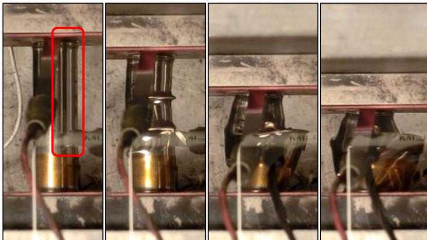
**Figure 1:** Cylindrical lithium-ion cell undergoing axial crush between two flat plates
