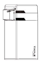
On the right side of BMS, after the charging cables (please refer to section 4.5.5) and CAN communication cable (please refer to section 4.5.3) are correctly connected, screw the terminal box small (J) with M4 srews and lock the terminal box cover (K) also with M4 screws. On the right side of battery module, screw the terminal box medium right (I1) with M4 screws and lock the terminal box cover (K1) in the same way as BMS. Please see the installation diagram on the right.
