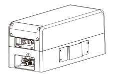
After the power cable has been correctly connected, and all RS485 communication cable (please refer to section 4.5.2) and ground wires (please refer to section 4.5.4) are correctly connected, lock the terminal box\_large(L) to the out side of BMS and battery module on the left with M4 screws(N).
